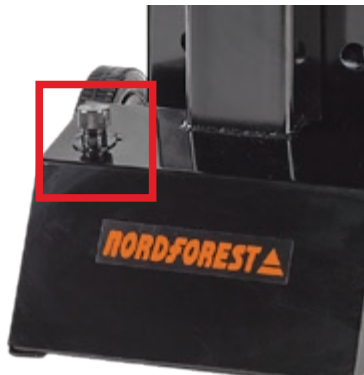
Fig. 9: Filling screw with dipstick
