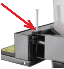
Fig. 3: Axis of rotation of the actuation arm
