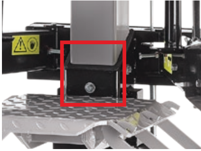
Fig. 8: Greasing the splitting column
